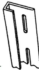
*Packing strip, inserted into slot of D5*
