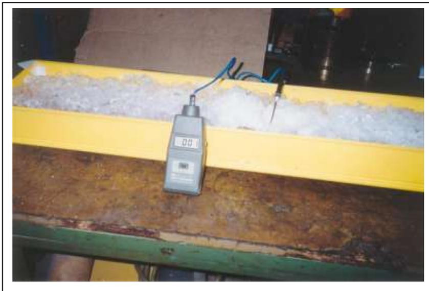
**Photograph #2.** *Digital Thermometer / Ice Bath Unit*
